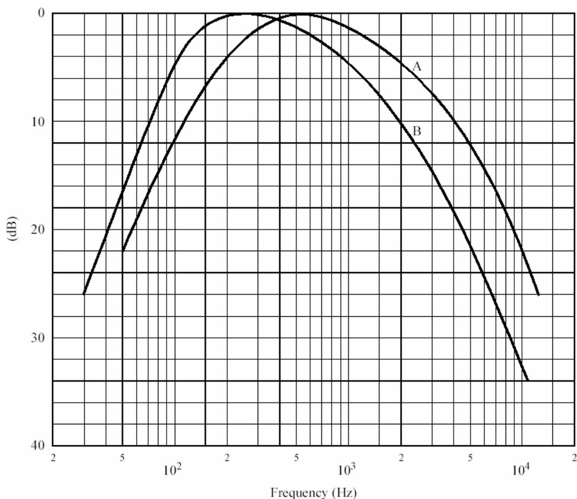
Curves A: frequency spectrum of standardized noise (measured with one-third octave filters)
