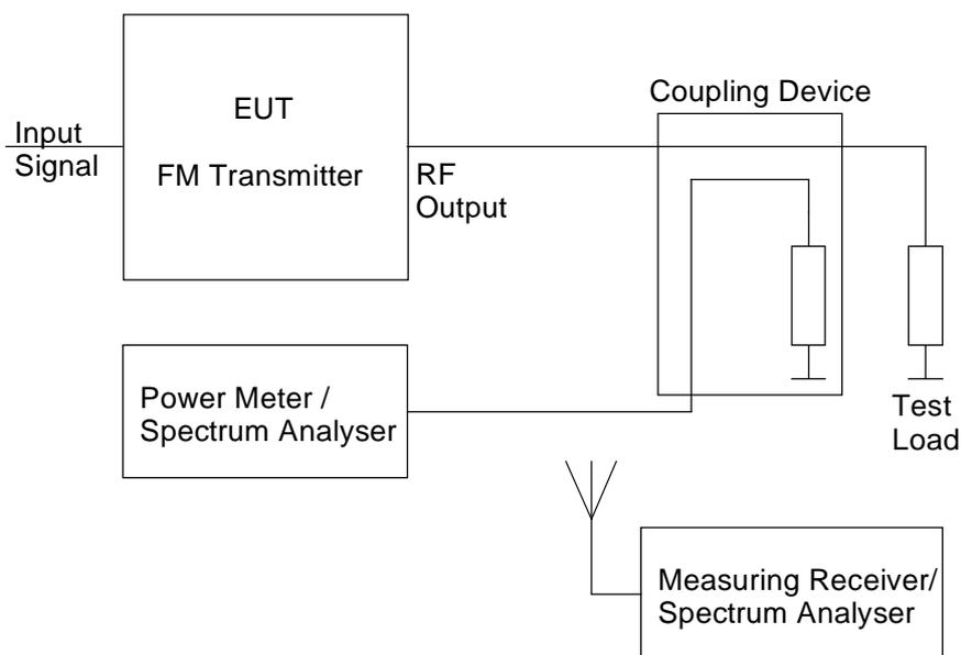
Figure A.5: Testing arrangement for cabinet radiation
