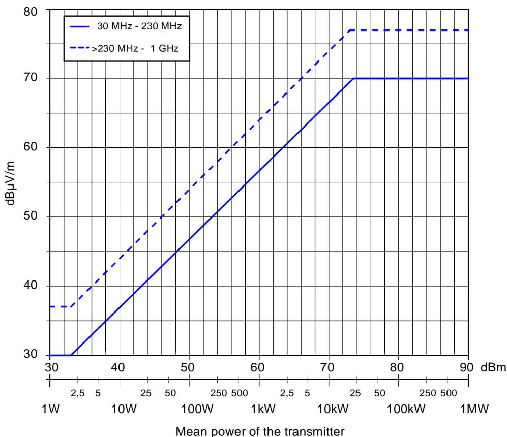
Figure 4.3: Cabinet radiation limits for FM transmitters
