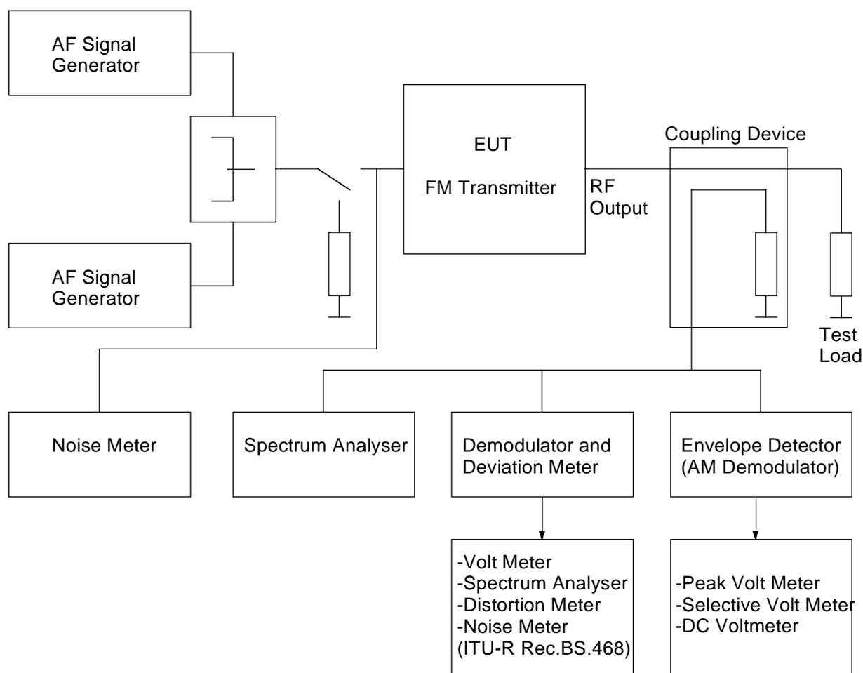
Figure A.1: Testing arrangement for monophonic transmitters
