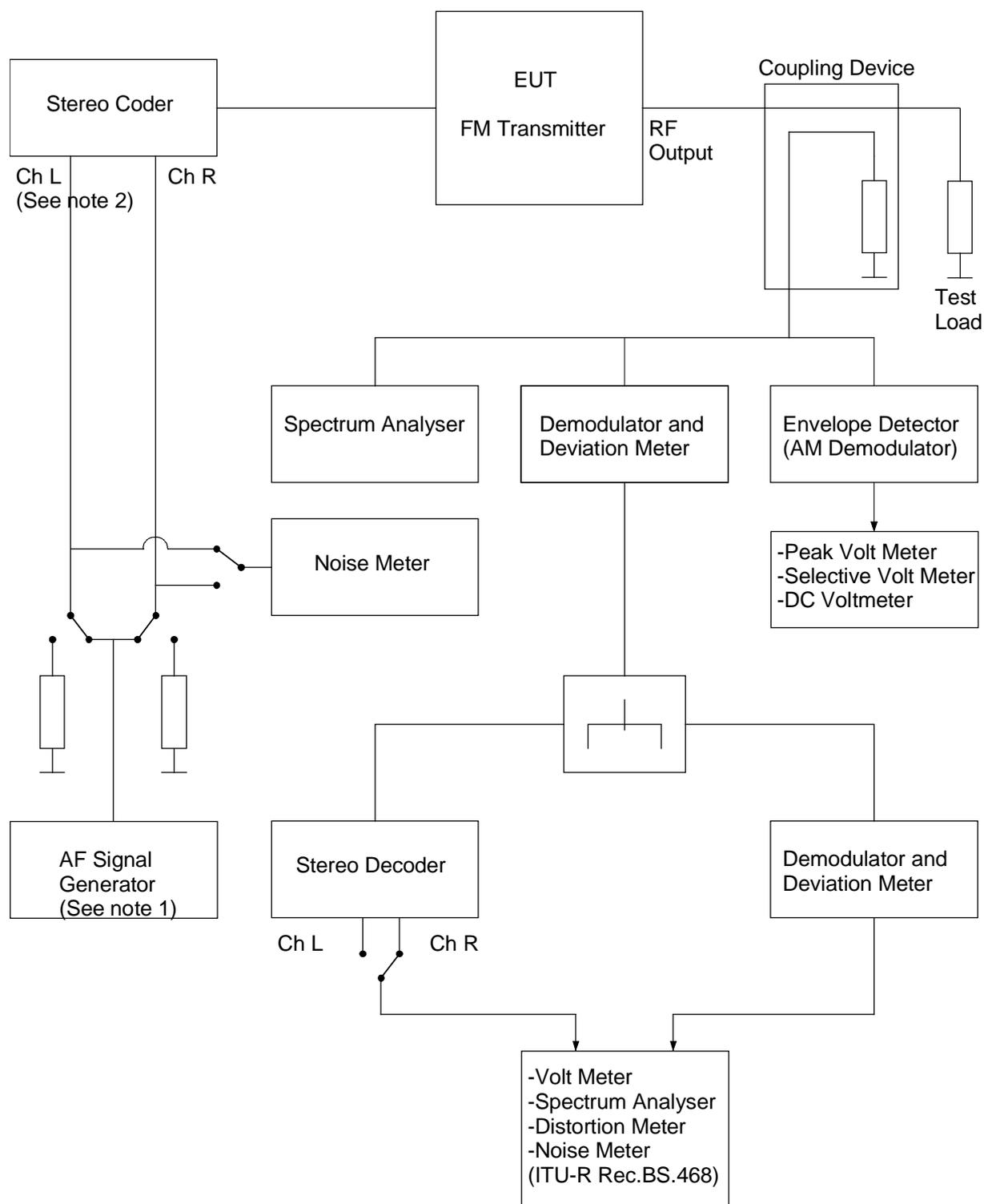
NOTE 1: AF Signal Generator is replaced by coloured noise generator when is requested.
