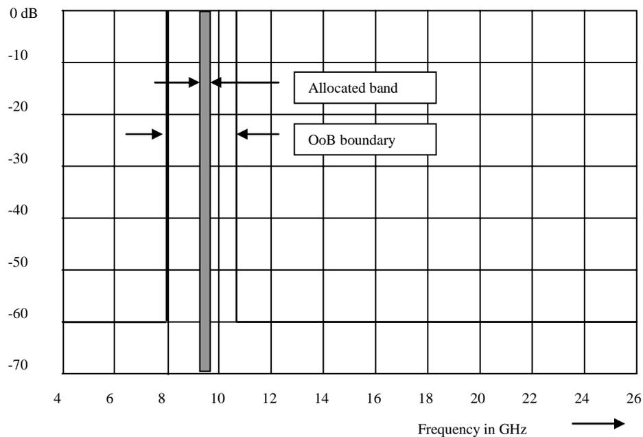
**Figure C.4: Maximum permitted spurious emissions power level**
