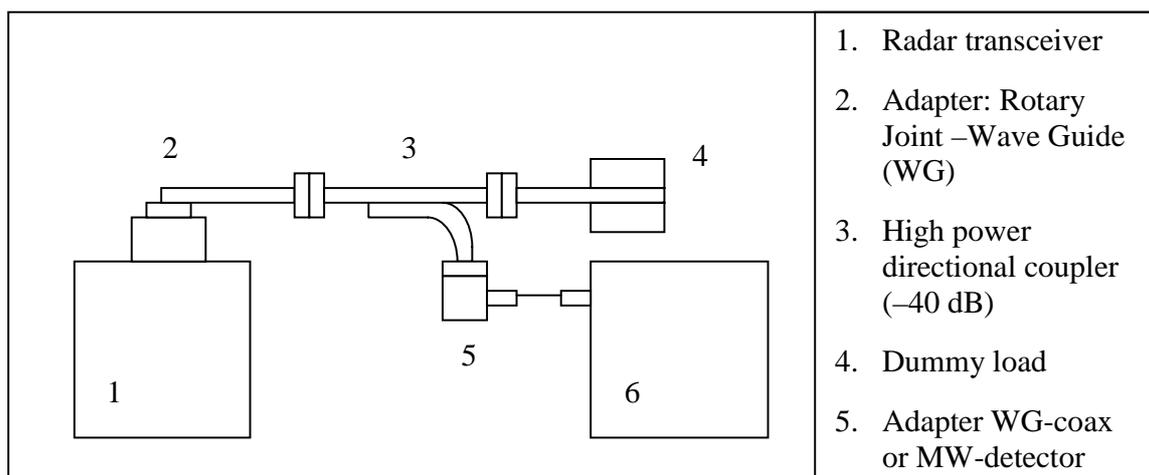
Figure C.1: Measurement of the operation frequency and the pulse power
