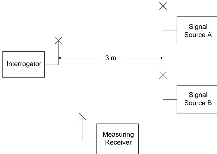
**Figure B.4: Radiated measurement of blocking**
