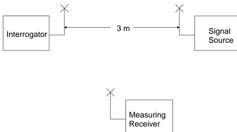
**Figure B.2: Measurement of threshold level**
