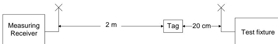
**Figure 6: Measurement of tag emissions**
