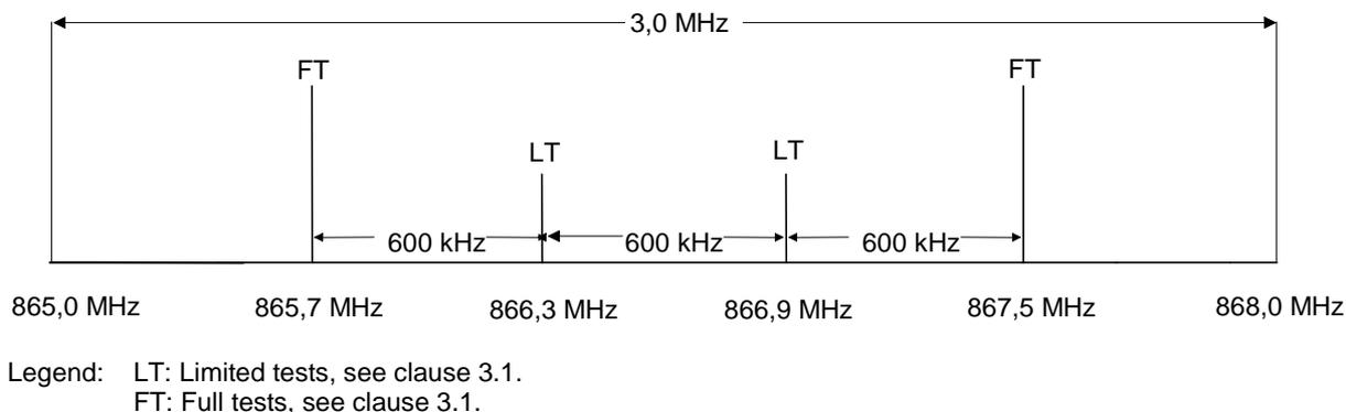
**Figure 2: Tests on a single sample for equipment within the band 865,0 MHz to 868,0 MHz**
