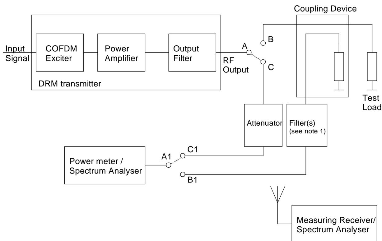
NOTE 1: Filter(s) not used in Rated output power measurements.
