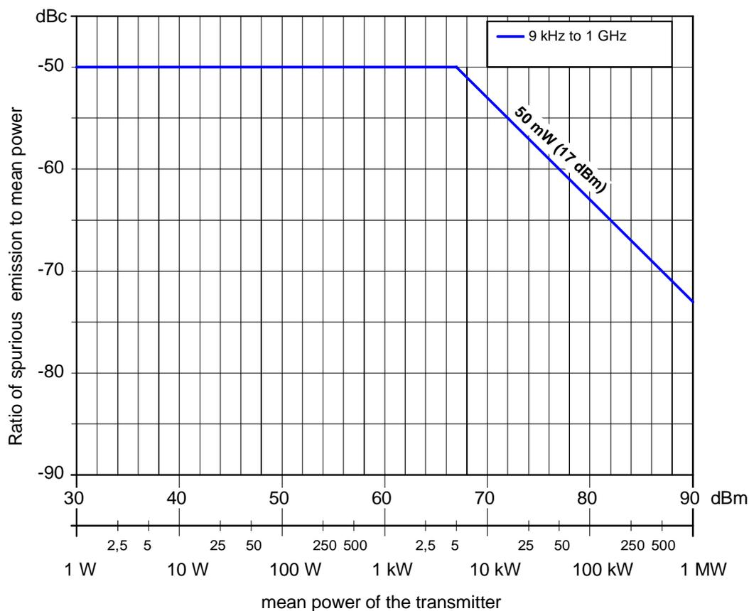
**Figure 4.1: Spurious emission limits for DRM transmitters**
