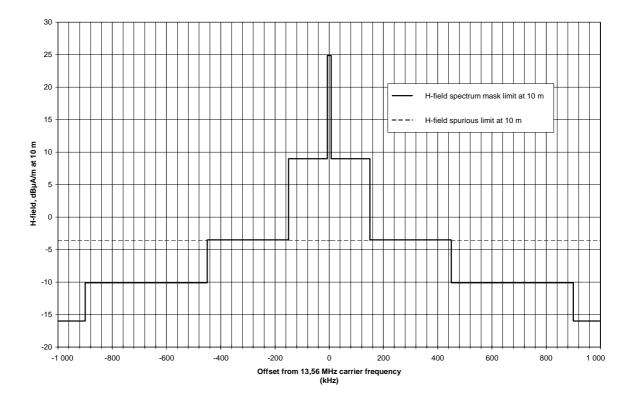
Figure 1: Transmitter spectrum mask
