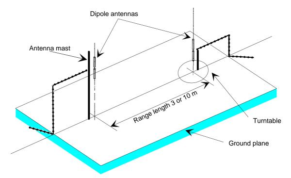
Figure A.3: A typical Open Area Test Site (OATS)
