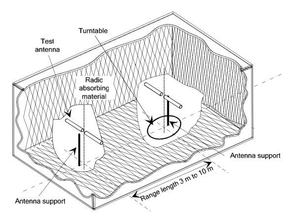
Figure A.1: A typical anechoic chamber
