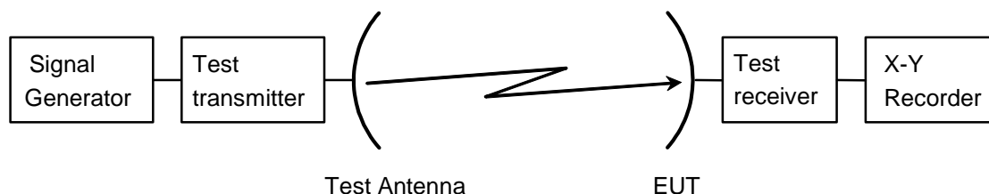
Figure 10: Test arrangement - antenna transmit radiation pattern measurement
