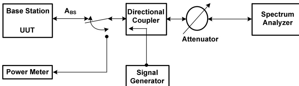
**Figure 5: Test Setup for BS transmitter intermodulation requirement**
