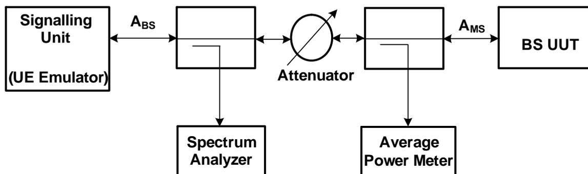
Figure 4: Test Setup for BS maximum output power
