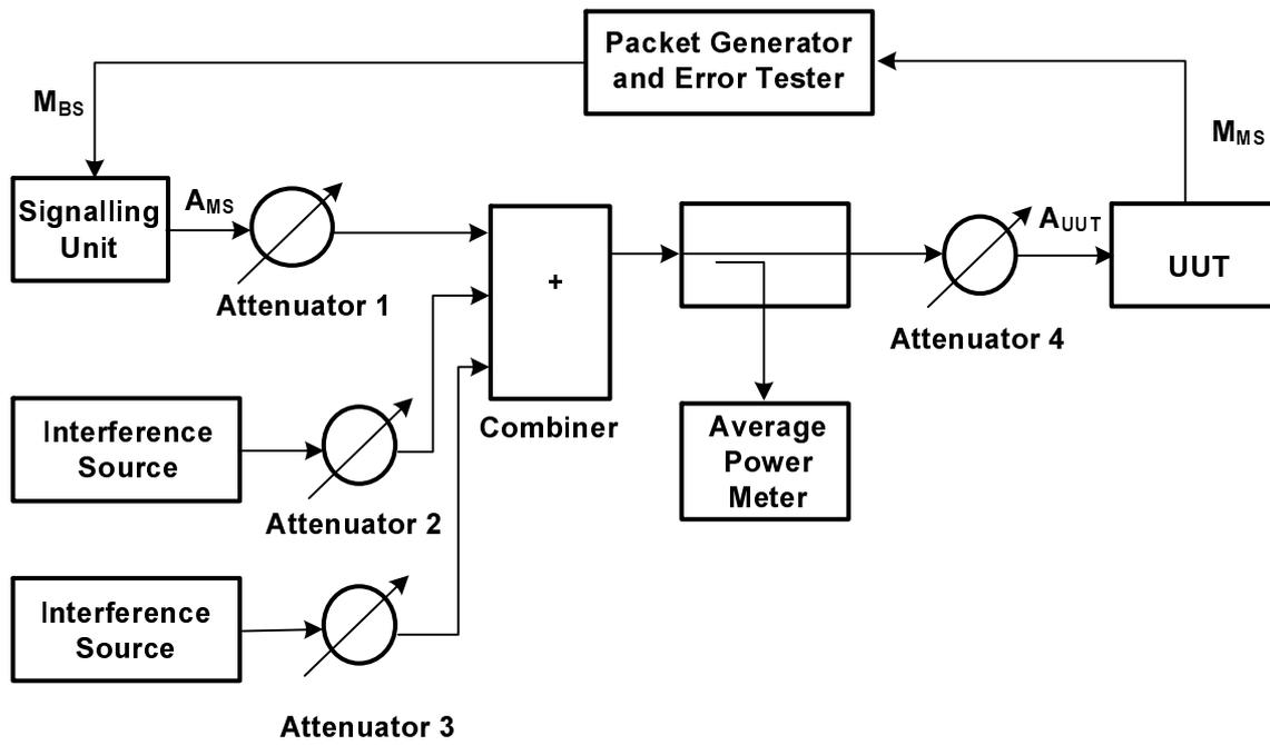
Figure 9: Test setup for receiver intermodulation test
