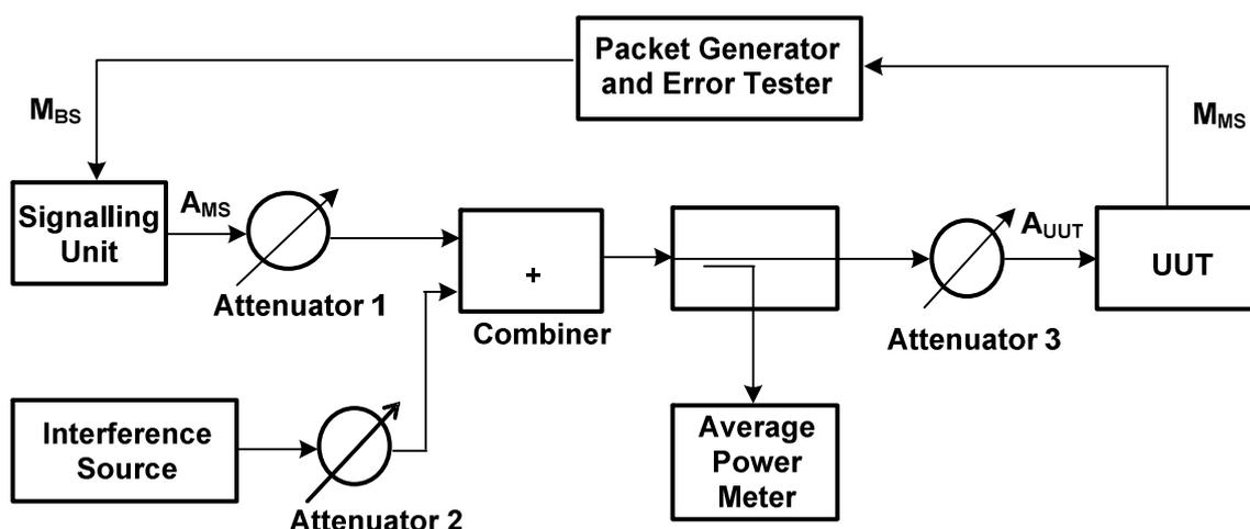
**Figure 8: Test setup for receiver blocking test**
