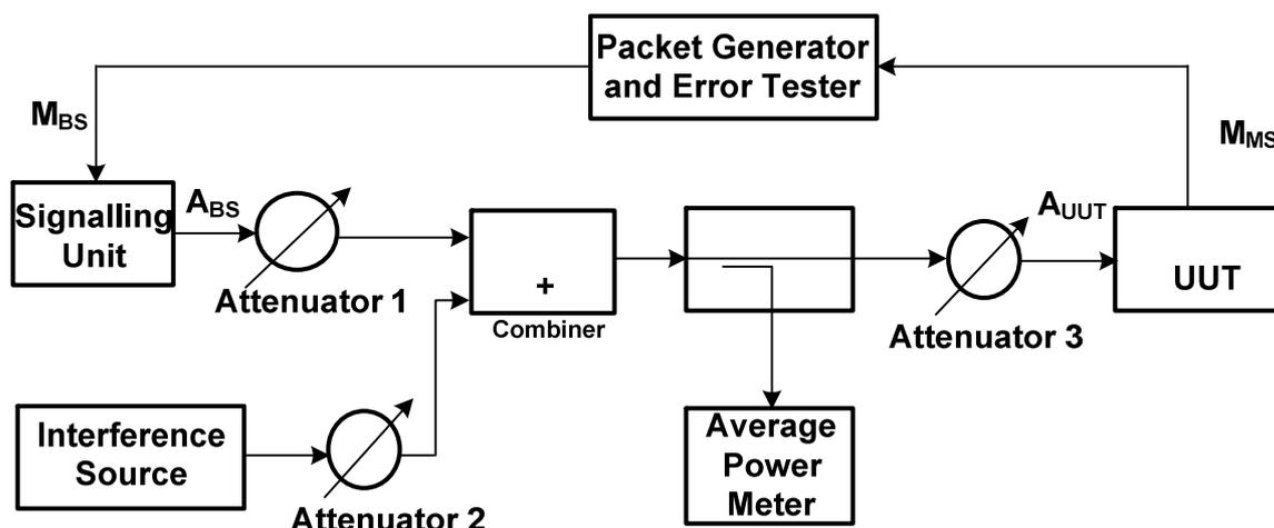
Figure 8: Test setup for receiver blocking test
