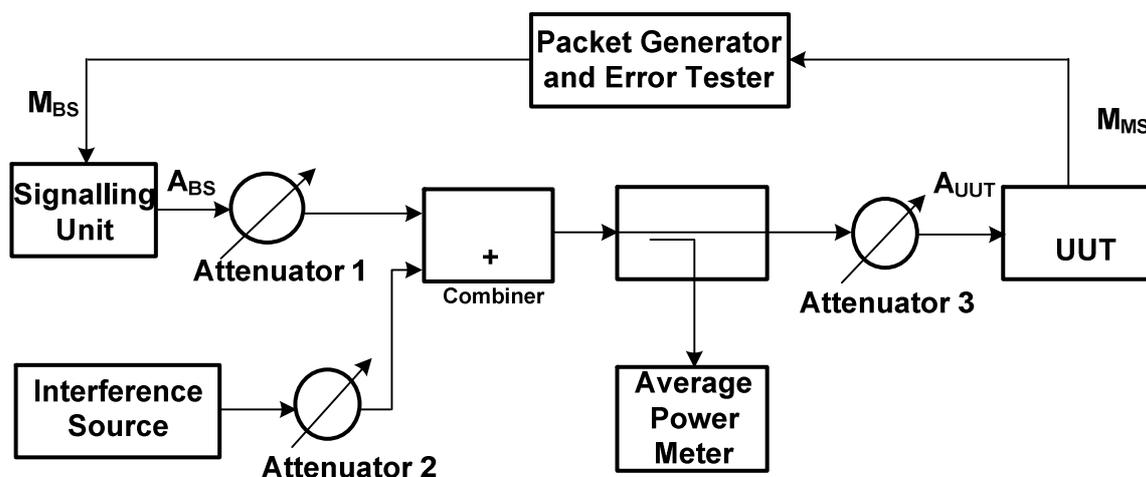
**Figure 10: Test setup for receiver spurious response test**
