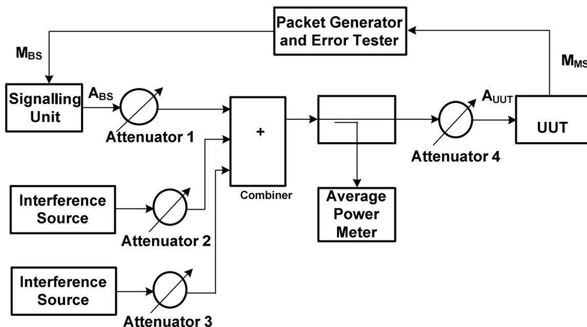
Figure 9: Test setup for receiver intermodulation test
