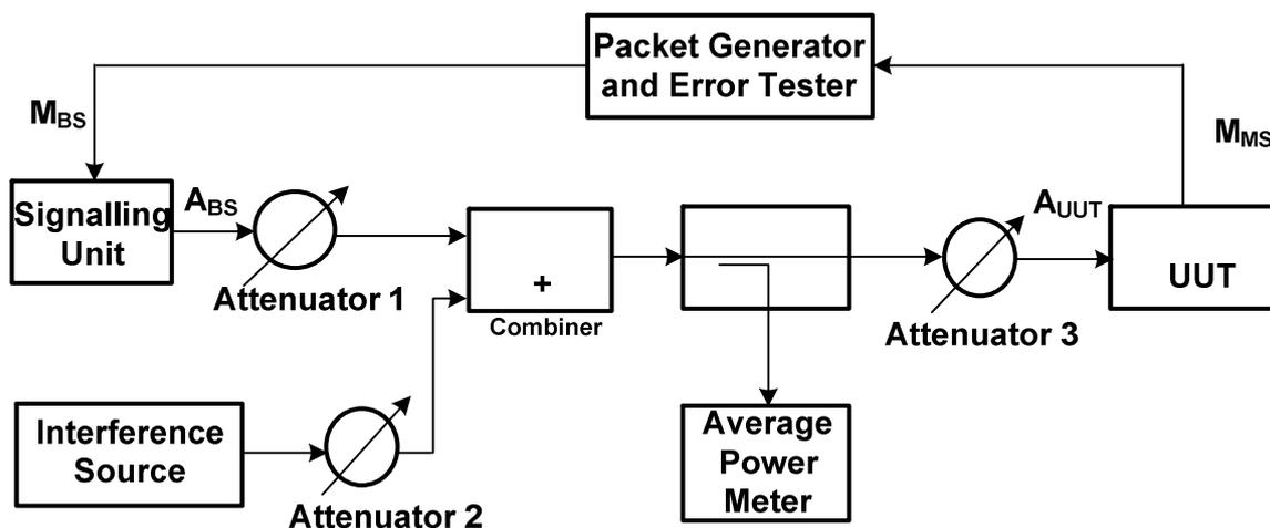
Figure 7: Test setup for receiver adjacent channel selectivity test
